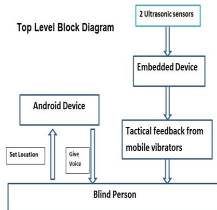
Fig.1.Top level block diagram
