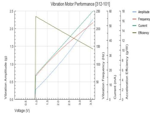
**Fig5: Characteristics of Vibrator Motor**
