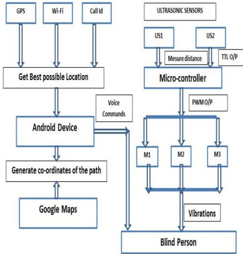
**Fig.2 System level block diagram**
