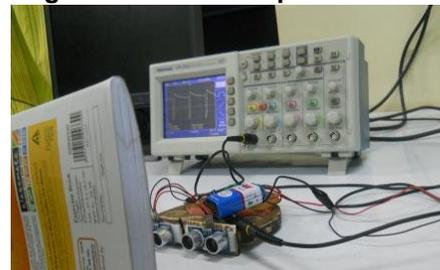
As stated before the final product is intended to be comfortable, light weight so we fabricated the housing of the embedded device using wood. We got the idea of this design from a knuckle punch. Further we have used a 9V Radio Battery with a TI's UA7805CKCS voltage regulator and a pair of AA batteries to power the MSP430G2553 with 3V supply and mounted batteries with a power switch. The final device without the app is shown in fig. 8
