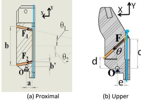
**Figure 4:** Cross sections of Proximal and Upper phalange showing Flexion Tendons (Orange) and Extension Tendon (Blue) and Tendon-Paths;  $F_1$  and  $F_2$  are the Tension in the Tendon at points shown.
