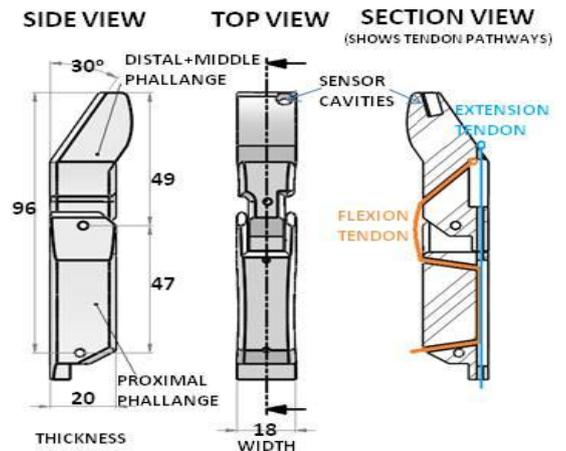
Figure 3: Index Finger Design showing various dimensions and sectional view with tendon paths.
