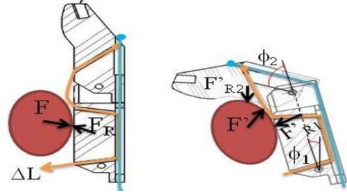
**Figure 7:** Adaptive grasping by a finger showing Flexion rotation angles and contact forces.
