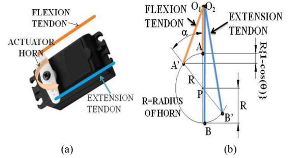
**Figure 5:** (a) Tendons fixed on the Horn; (b) Schematic representation of the Tendon-Horn system.
