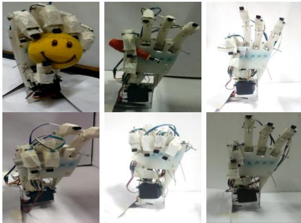
Figure 10: Various Grasps performed by the Robotic Hand.
