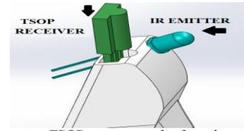
Figure 8: Mounting TSOP receiver and infrared emitter on tip of a finger.
