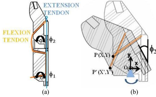
**Figure 6:** (a) Tendon Pathways and Rotation angles  $\phi_1$  and  $\phi_2$  for two phalanges; (b) Rotation of Upper phalange by  $\phi_2$ .
