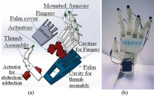
Figure 9 : (a) Exploded CAD View of the Hand Assembly.
